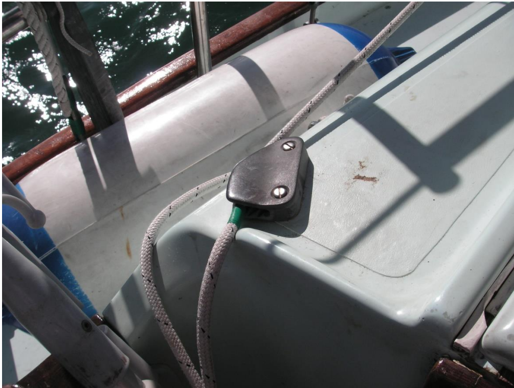
The Clam Cleat with the green tape marking the position for the roving pulley
