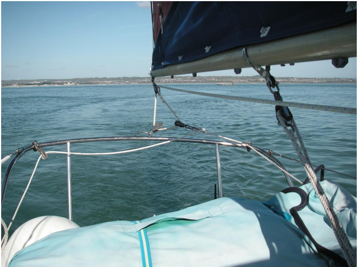
The mizzen on a port tack set with the rope traveller and roving pulley
