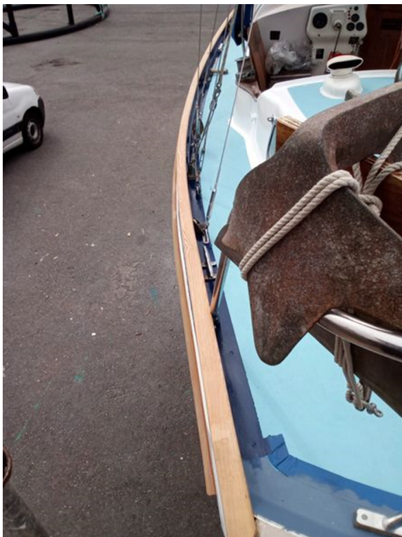
Port-hand toe-rail complete
