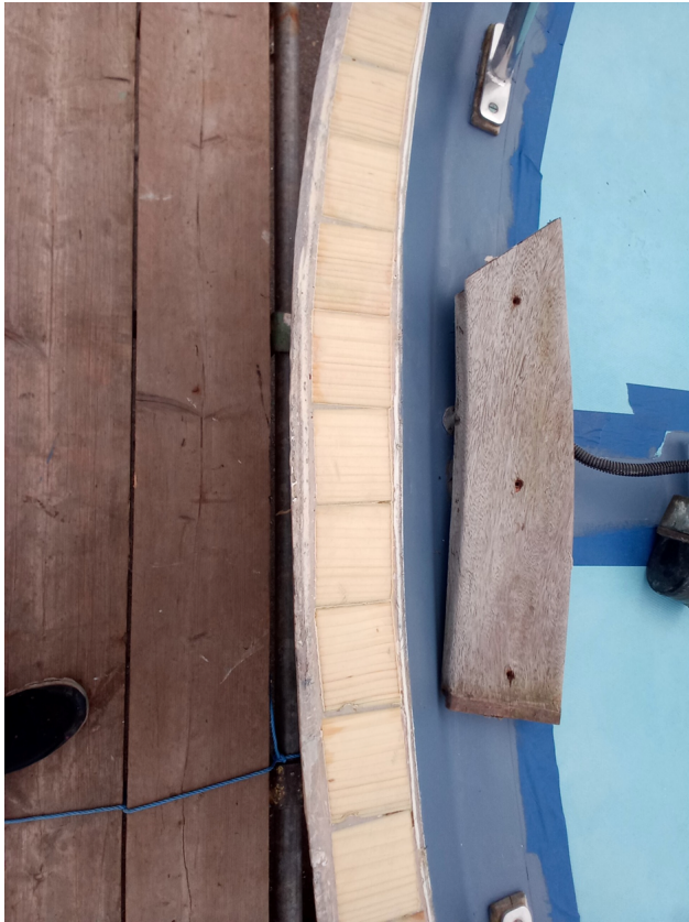
Stern sanded fair together with a section of the original toe-rail
