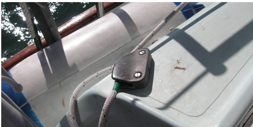
The Clam Cleat with the green tape marking the position for the roving pulley
