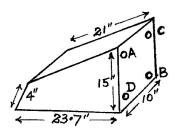
There are four tappings to the calorifier – A and B going to the heat-exchanger coil – although 'square' would be a better description – it being made from Yorkshire elbows and 22mm copper pipe. Hot water in at A and return to engine at B.
