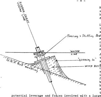
He had had a serious and expensive leakage and had fitted a heavy sub-flange of brass screwed down with \*umpteen\* wood screws.
