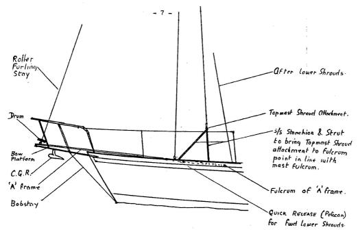
release, pelican type hooks. Both masts are lowered together and from the photos the roller forestay is then nearly horizontal and the 'A' frame at about 70° Lowering fully for lifting off is of course only an extension of this procedure.
